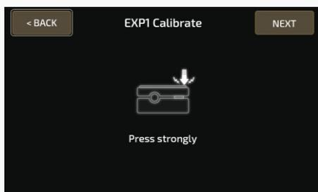
Then, strongly press the pedal toe down and press NEXT. The calibration will be set, and this message will appear:
