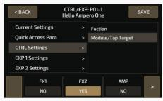
The 9 Ampero One effects modules are listed in the panel, with yes and no below each module to show if the CTRL footswitch is activated or not. In the example image above, FX1 and FX2 are controlled by the CTRL footswitch, whereas the AMP module is not. Slide (or use Main Knob) to change between yes/no, and press the arrows on the right/left to scroll through the modules.
