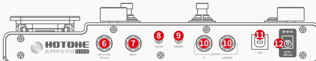
**6. EXP2/CTRL:** 1/4" TRS input, for connecting an external expression pedal. Perfect for Hotone Ampero Press or Ampero Switch.
